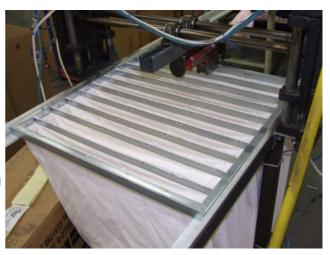
The filter material construction consists of pockets which are ultrasonically welded, cut to size and supported by a corrosion resistant metal or plastic frame.
